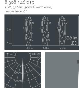
Customized solutions and modifications are possible: Special RAL, DB or NCS colours as polyester powder coat, luminaires in 2700 K and other colour temperatures and versions for high ambient temperature.
